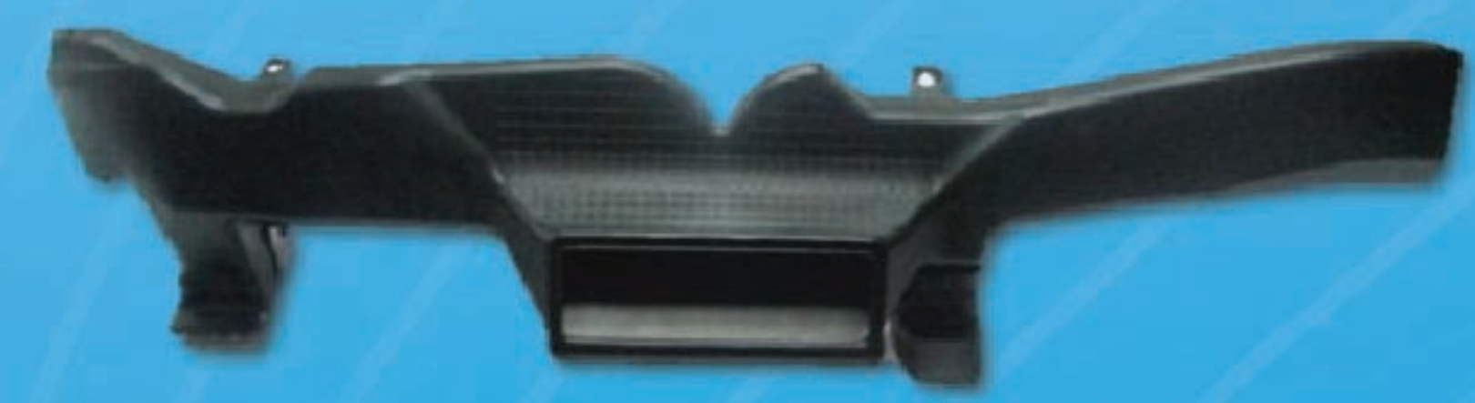
DUCT HEATER TO REGISTER CTR
